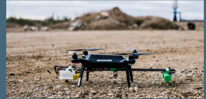
Drones mounted with laser sensors to detect methane emissions
