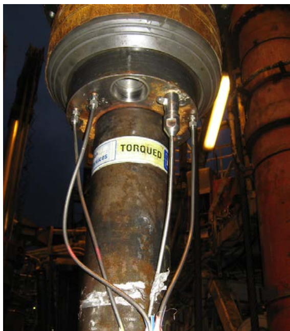
Figure 3-6 Photo showing the control lines coming from valves, entering the tubing hanger (seen from below tubing hanger)
